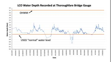
Volunteers regularly monitor the depth gauge at the Thoroughfare bridge. The gauge and the chart readings are in tenths of a foot (1/10 foot = 1.2 inches). The first point on the chart, June 27, 2017, was when the gauge was first installed. The gauge was moved to the upper end of the bridge abutment on 4/15/21. The USGS "normal" water surface elevation for big LCO is 1287 feet and is represented by the lower orange line.
